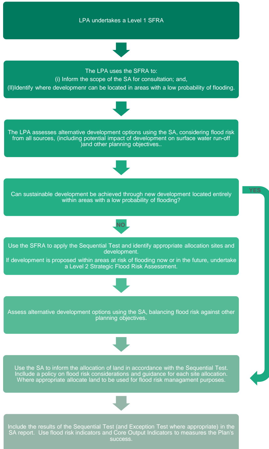
Figure 1-1 Taking flood risk into account in the preparation of strategic policies (PPG Flood Risk and Coastal Change Diagram 1)
